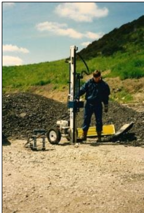
Hand Portable Dynamic Probe and Sampling Rig (50kg weight with 500mm free-fall)
