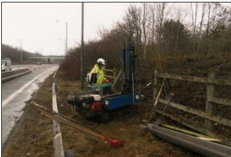
Soil testing to aid foundation design for proposed overhead signage on M56 Motorway by terminal 2 Manchester Airport.
