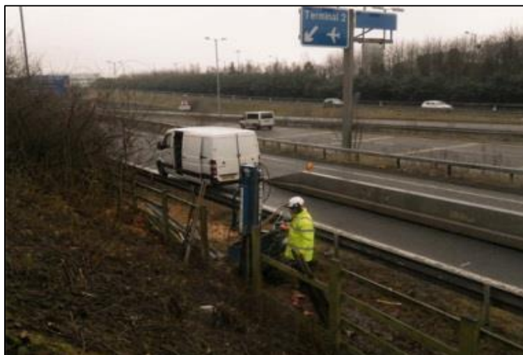
Soil testing to aid foundation design for proposed overhead signage on M56 Motorway by terminal 2 Manchester Airport.
